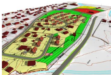
A planned housing development, shown both on a background of maps and plans, and an ortho photo draped over the modeled terrain.
